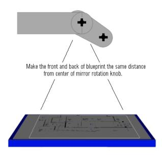
**<u>IMPORTANT:</u> DO NOT OVER-TIGHTEN THE KNOBS** !!! JUST MAKE THEM FIRM ENOUGH TO PREVENT MOVEMENT. Fine Tune Front to Back Adjustment
